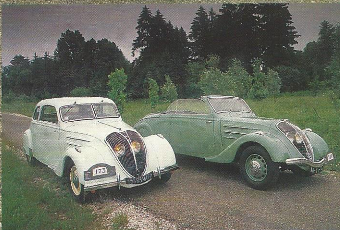
Eclipse models its retractable roof; car is a 402, and not a later 402B. Alongside is 402 coach from 1936 - but wearing grille from a 402B. Unlike the coach body on 402B, car has centre pillars rather than pillarless hardtop roof. Confused? Complex range is unscrambled on final page
