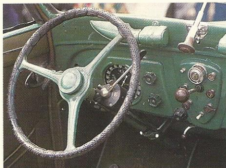
Driving compartment of coach : note dash-centre push-pull gearchange – Portuguese car uses Cotal 'box with steering-column control lever
